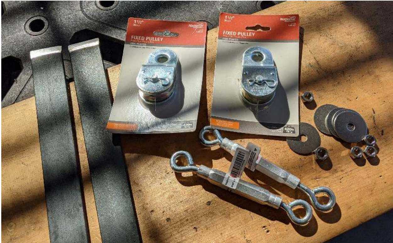
Caption below ↓ – The sharpened edge steel bar stock and materials for the under bucking tool wheel made from 5/16-inch turnbuckles, flat washers, nuts, and pulley wheels
