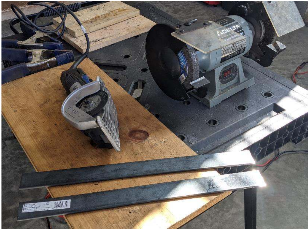
Caption below ↓ – Second step, file the chisel point ends of the steel bar stock to a sharp edge like sharpening an axe
