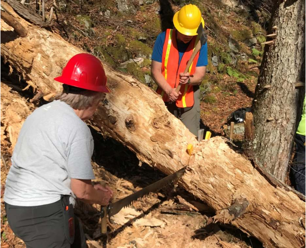
Caption Below ↓ – Wedges set in large oak log to overcome top and side bind, aluminum wedges with additional plastic wedges were necessary to lift the log and keep kerf open for successful top cut, Three Ridges Wilderness, Virginia
